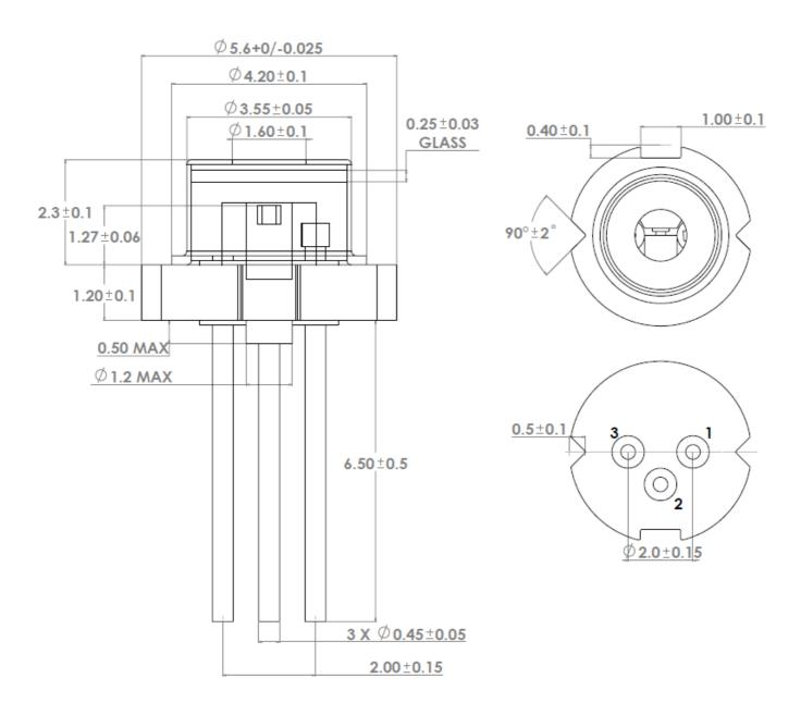
Note: Tolerance is ± 0.05mm for items without tolerance marking
