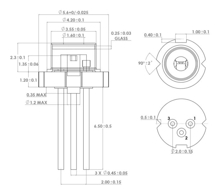
Note: Tolerance is  $\pm 0.05$ mm for item without tolerance marking
