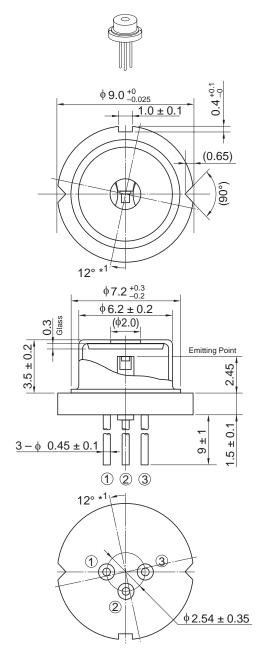
Note: 1. The beam has 12 deg offset against the package reference plane. Please take account it mounted on a board.
